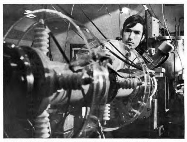
VAN DE GRAAFF ACCELERATOR BEAM is adjusted by Tom Picraux (5111) to send ions down a specific lattice channel in order to study the effects of ion implantation as a method of "doping" semiconductors.
